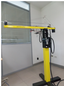
FIGURE 2 – Lab sized tower crane
